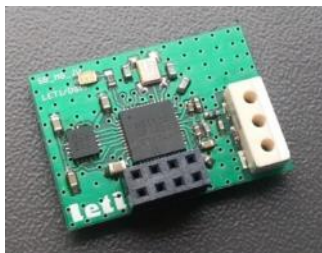
Low-Power Bluetooth Low Energy & 868MHz Platforms 200\mu\text{J} - 600\mu\text{J} / measure+emission
