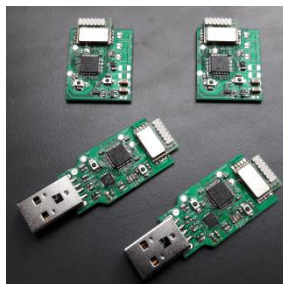
Low-Power Bluetooth Low Energy & 868MHz Platforms 200\mu\text{J} - 600\mu\text{J} / measure+emission
